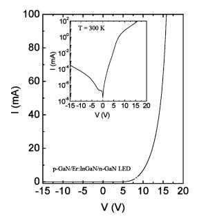
FIG. 2. I-V characteristics of a p-GaN/In\_{0.05}Ga\_{0.95}N:Er/n-GaN LED. The inset shows the same plot on a semilog scale. The leakage current is  ${\sim}0.2~\mu m$  at  ${-}15$  V bias.
