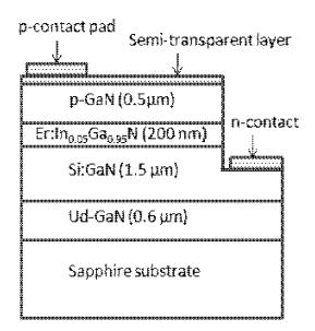
FIG. 1. Schematic of the multilayer structure of the fabricated p-GaN/ Er:InGaN/n-GaN LEDs. The active region is a 200 nm thick Er doped In<sub>0.05</sub>Ga<sub>0.95</sub>N epilayer [or (Er:In<sub>0.05</sub>Ga<sub>0.95</sub>N)].
