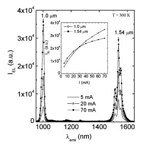
FIG. 5. Near IR EL spectra of a p-GaN/Er:  $In_{0.05}Ga_{0.95}N/n$ -GaN LED under different levels of injection currents. The inset shows the peak EL intensities of 1.0 and 1.54  $\mu$ m emissions as functions of injection current.
