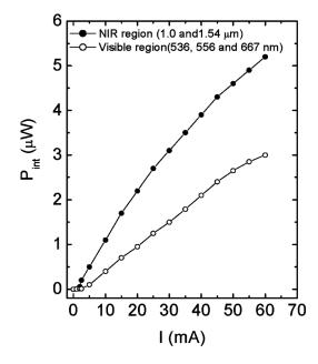
FIG. 4. Integrated optical power, over the visible and near IR regions, of a p-GaN/Er:  $In_{0.05}Ga_{0.05}N/n$ -GaN LED as a function of input forward current.
