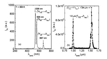
FIG. 3. RT EL spectra of a p-GaN/Er: $In_{0.05}Ga_{0.95}N/n$ -GaN LED (a) in visible region, and (b) in near-IR region under a current injection of 20 mA with a forward bias of 12.5 V.
